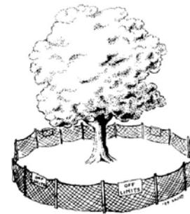
**Figure 2.** Protect the tree from damage by erecting construction limit fencing around the protected root zone.
